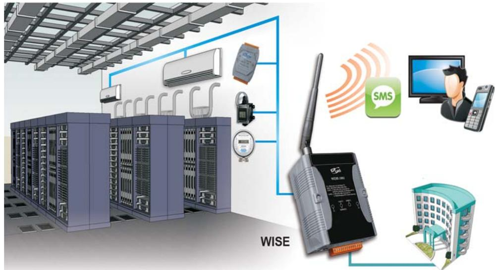
In addition, it allows to connect to WISE controller by SCADA software to perform the control, monitoring and collection of the I/O channel data of the facilities. And the power consumption of facilities in the control room can be statistically calculated in order to manage the electricity usage and cost as well.
